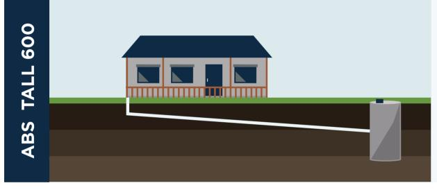
Invert Height 1,270mm Total Drainage Run Up to 40m Depth In Ground 2,900mm
