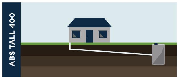
Invert Height 1,070mm Total Drainage Run Up to 22m Depth In Ground 2,700mm **Emergency Storage** 5,182L (3.5 days)
